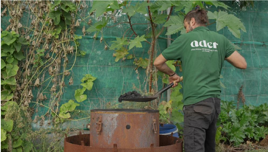
Image 14. Production of biochar for the improvement of degraded agricultural soils.
